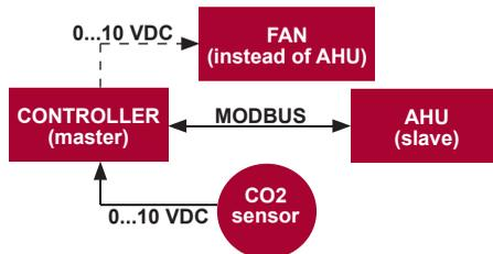
This controller allows controlling level of carbon dioxide (CO2) in a room. Connect 0..10VDC CO2 sensor directly to the controller and configure the controller. In service mode, in item F.14 set 2, and F.15 and F.16 should be set based on the sensor specification.
